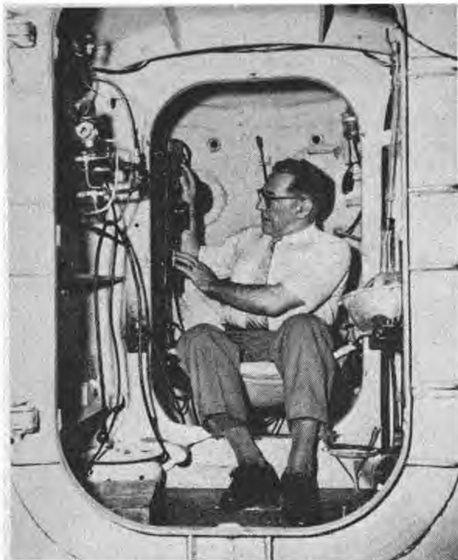
Inside Space Cabin Simulator, photographed through open door. Behind author's head is small airlock for passing meals into cabin
