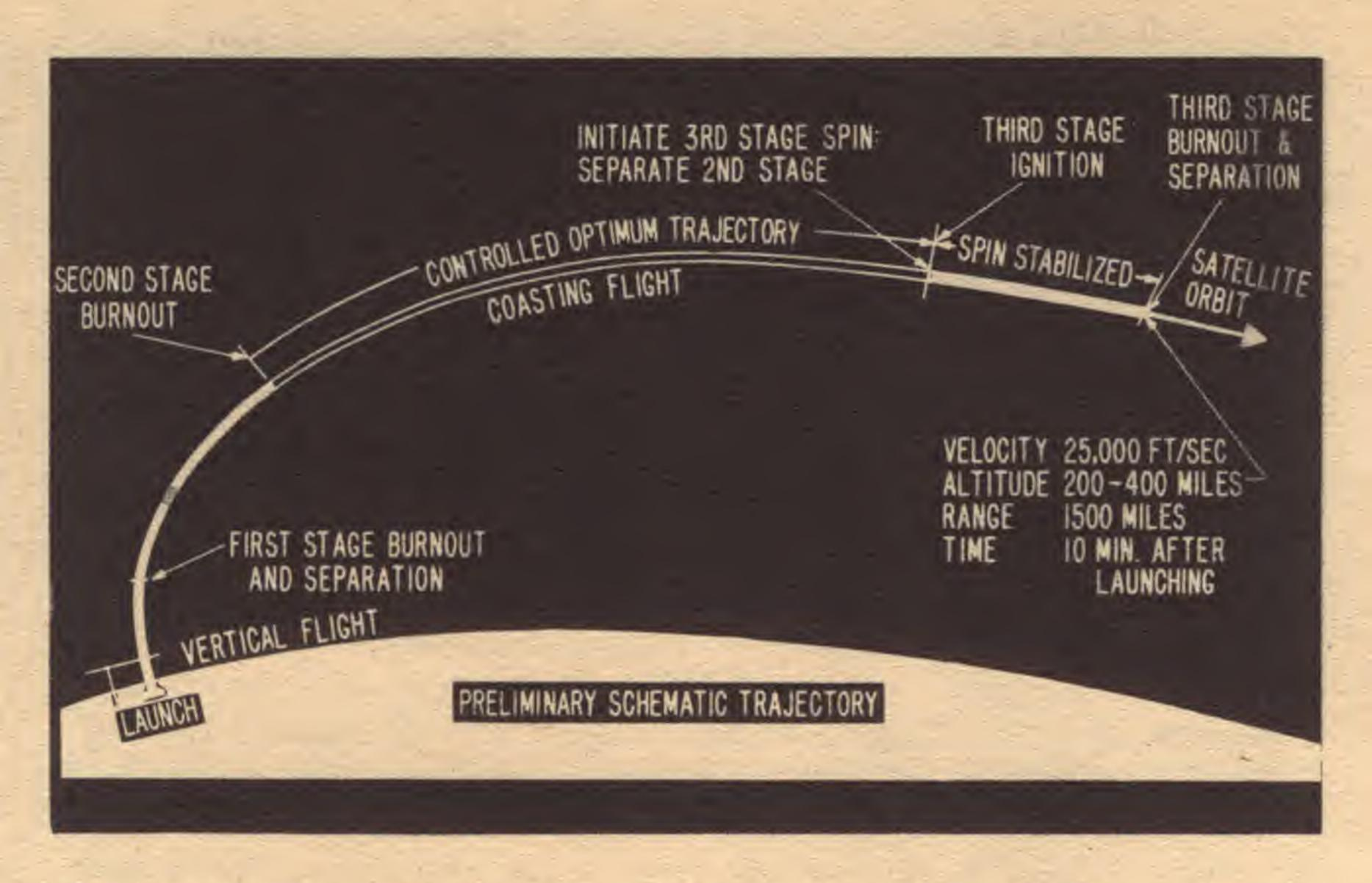
The official schematic drawing of the satellite shots. The term "range 1500 miles" on the diagram refers to the expected impact point of the second stage, about 1500 miles from the takeoff site.
