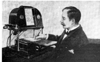
The telautograph will transmit messages in the actual handwriting of the sender.
