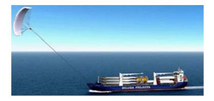
Kite sails are still quite experimental, but in 2008 the M/V Beluga Skysails made a 12,000 mile round trip using a computer-controlled 160 square meter towing kite, deployed at an altitude of 100-300 meters, to save about 10-15% in fuel cost. Its kite sail is supposed to operate at winds of Beaufort Force 3-8, and it can tow the ship as close as 50 degrees to the upwind direction. (Skysails).
