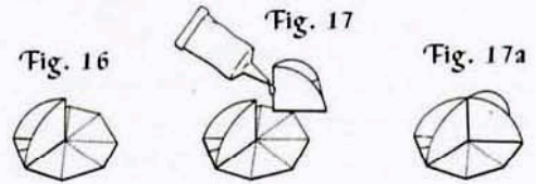
FIGS 17, 17A. Glue part 39 to the opposite segment indicated, also gluing the folded edge so that 38 and 39 are glued together.
