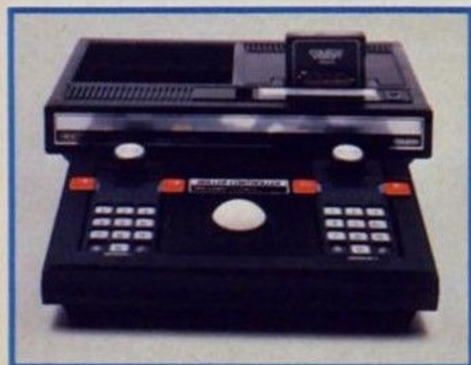
Below: ColecoVision's latest control console, Roller Controller has a track ball that gives the player 360-degree free-rolling movement and greater momentum for onscreen action, about $60, including Slither, a video-cartridge game that pits the player against a desert world. It attaches to the ColecoVision console, $180.
