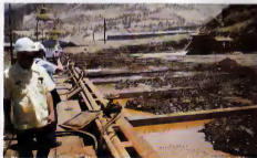
Copper ore dissolved in water by microbes is precipitated over iron bars to extract pure copper.
