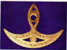
This brass quadrant, made in 1588, was used to measure height of heavenly bodies above horizon.
