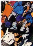
Micro-twin section of moon rock reveals aluminum, iron, titanium, and magnesium-iron materials for future construction.
