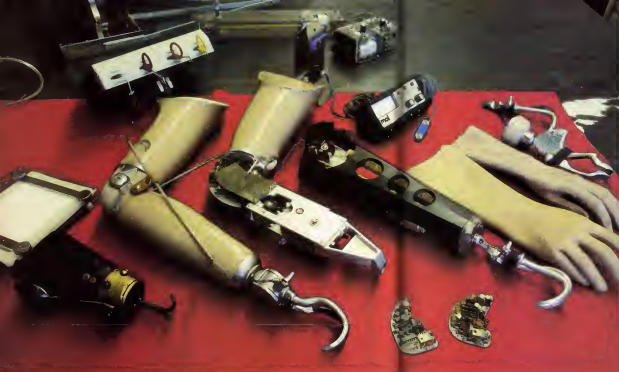
Above: Array of artificial arms shows a history of the phosphenes. At top left is 1968 model. Electronic parts in background are amplifiers for picking up electrical muscle signals. In two photos at right, top arm center, Dr. Stephen Jaccubson, father of the Utah arm, shows how it responds to signals. Sensor is clipped to his left forearm. When he raises his hand, the arm rises also. Far right: Modern hand compared to 1968 hook. Near right: The tiny Strykeprobe blood sensor
