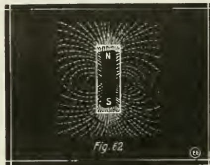
Fully Developed Magnetic Field of Force Around a Bar Magnet. The Greatest Strength of Field is Manifested at the Ends of the Bar, Where the Flux is Most Dense.
