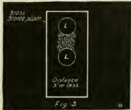
Peculiar Form of High Tension Discharge Obtained Between Two Leyden Jars Set on Brass-Bronze Paper.
