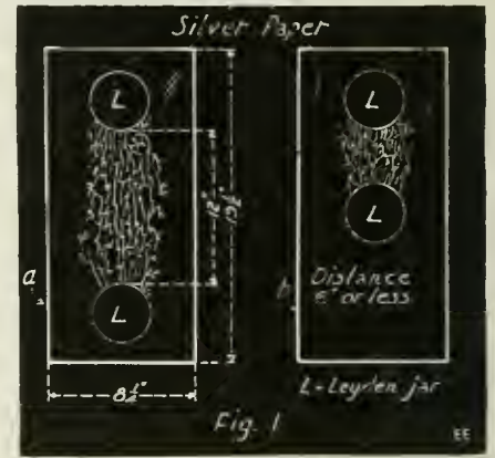
Spectacular Condenser Discharges Can Be Arranged With Metalized Paper, a Pair of Leyden Jars and a Small 3" Static Machine. This is a "Silver Paper" Experiment.
