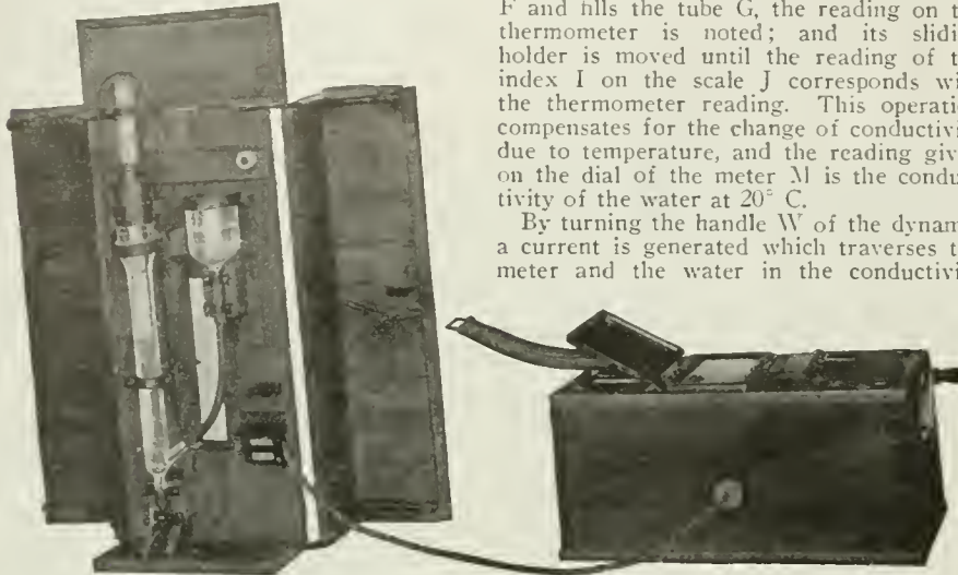
General Appearance of New Dionic Electric Water Tester. Operates on the Principle that Relative Chemical Make-up of Water and Its Electrical Conductivity Correspond.
