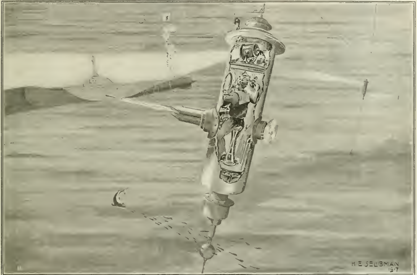
"Why Not Mine Harbor Approaches and Other Shallow Waters with a Series of Submarine Forts Like Those Here Shown?" Asks a New York Inventor. They Would Carry Powerful Sub-sea Searchlights, Microphones, Telephone (Connecting with Shore Station), and Special Torpedo Tubes for Torpedoing the Enemy Submarines, Should They Come Within Range.
