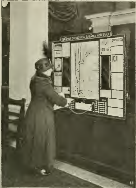
How Do I Get to 125 Street and Seventh Avenue? That and Hundreds of Similar Ones Are Now Answered by the Electric Street Guide, Here Shown Installed in the Hotel Martha Washington, New York City.
