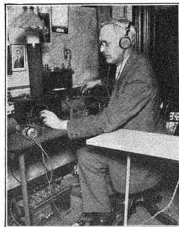
Lower Photo Shows Mr. Apgar in the Act of Actually Recording a Long Distance Radio Message on a Phonograph Cylinder. This "Canned Wireless" Has Helped Uncle Sam Immeasurably.
