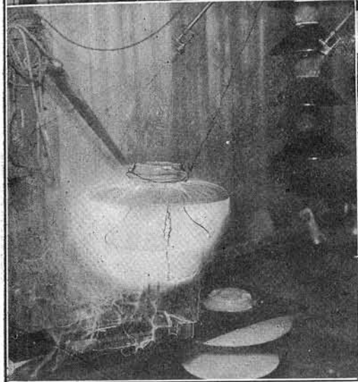
Fig. 3. Testing Electricians' Gloves Under Several Times the Voltage They Are Rated At.
