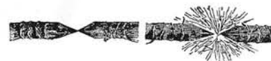
Showing the Effect of the Union and Separation of the Charcoal Points.
