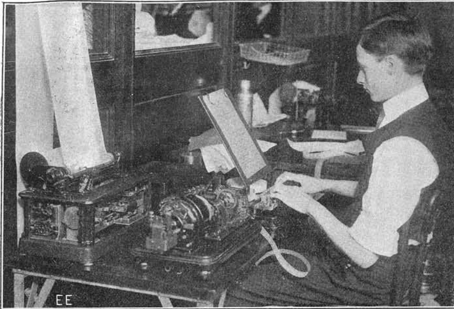
Photo (C) by Underwood & Underwood. Showing Morkrum Sending and Receiving Printing Telegraph System Installed in Associated Press Offices in New York City. Local Printer to Left.
